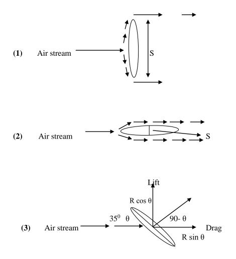
The reaction resulting form the diversion of air stream about a moving air born object may expressed by the equation
